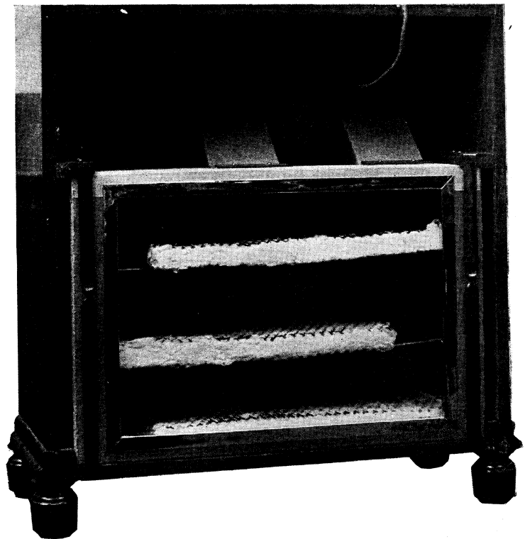
Acoustical labyrinth with back removed
